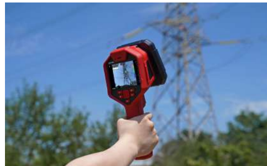
Partial Discharge Diagnostics
